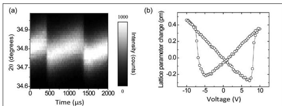
**Figure 3.** (a) Piezoelectricity-induced angular shift of the 002 Bragg X-ray reflection of a  $\text{Pb}(\text{Zr,Ti})\text{O}_3$  thin film in a bipolar applied electric field. (b) Piezoelectric hysteresis loop derived from (a). These measurements allow the local coercive electric field and piezoelectric coefficients to be measured.<sup>12</sup>
