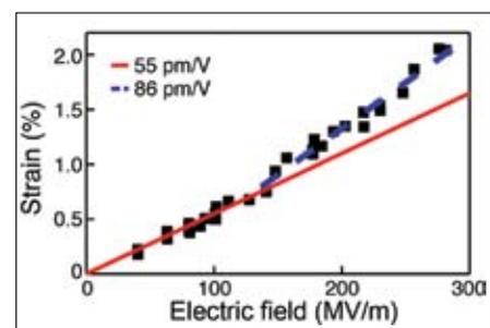
Figure 5. Electric-field dependence of the piezoelectric strain in BiFeO<sub>3</sub> thin films at very high electric fields. The low-field piezoelectric coefficient of 55 pm/V does not provide a good fit to strains observed at fields above  $\sim 150$  MV/m.<sup>11</sup>
