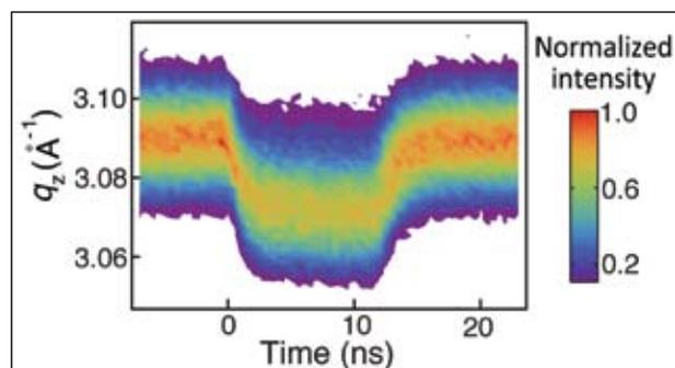
**Figure 1. Piezoelectric shift in the wavevector of the 002 Bragg reflection of an [001]-oriented BiFeO<sub>3</sub> thin film during an electric-field pulse lasting 12 ns. The wavevector shift corresponds to a piezoelectric strain of ~0.5%.<sup>11</sup>**
